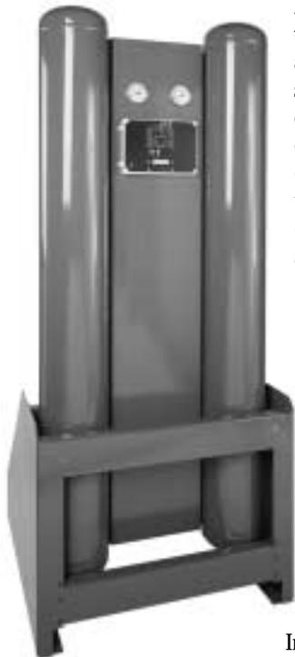
Regenerative desiccant type dryers normally are of twin tower construction. One tower dries the air from the compressor while the desiccant in the other tower is being regenerated after the pressure in the tower has been reduced to atmospheric pressure. Regeneration can be accomplished using a time cycle or on demand by measuring the temperature or humidity in the desiccant towers or by measuring the dew point of the air leaving the on-line tower.
